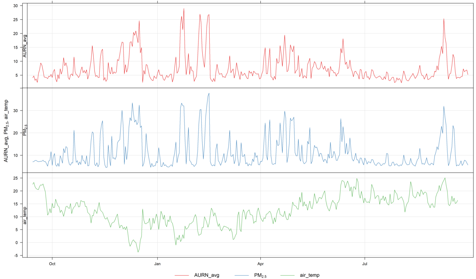
Figure A2.5: Time series plot of daily mean PM 2.5 concentrations (µg/m 3 ) at Z1142 (blue), average AURN PM 2.5 concentrations (µg/m 3 ) (red) and temperature (at Zephyr) (°C) (green), September 2022 to September 2023
